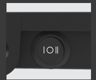
CCT switch located at the bottom
